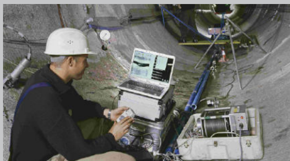
Borehole logging, rock laboratory
