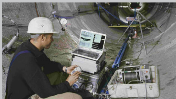
Borehole logging, rock laboratory
